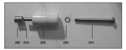
6. Inspect surface of plunger pipe (29B) carefully. Remove any chemical or mineral deposits taking care not to damage the surface of the plunger. If plunger pipe is worn, remove the plunger bolt (29C), plunger pipe (29B) and spacer (29E). Replace worn parts necessary. Note: <u>Always</u> use a new copper gasket (29) when repairing the plunger assembly.
